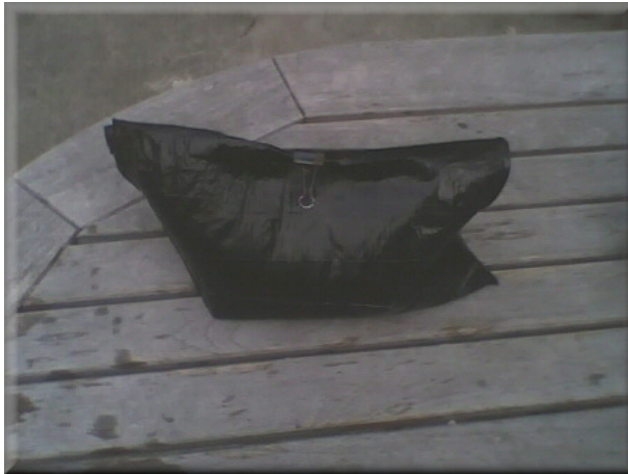
Figure 5. Joey bag – filled, compacted and clipped.
