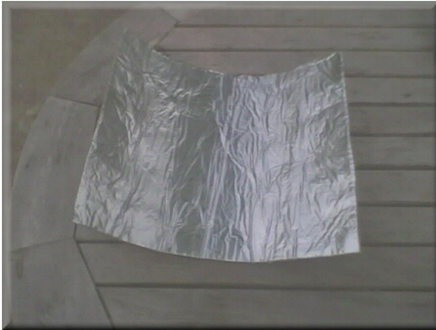
Figure 3. Solar cradle made from duct insulation, aluminum foil and clear plastic contact paper.
