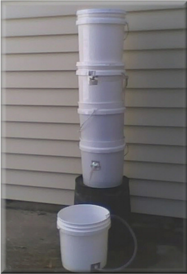
Figure 1. Modular BioSand Water Filter (prototype).
