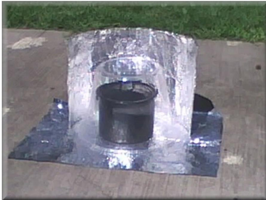
Figure 1. PanCooker - a solar thermal cooking and water pasteurization tool.
