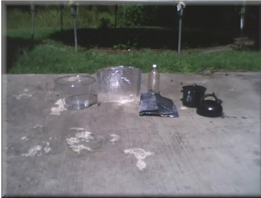
Figure 2. PanCooker components - from left to right: 12-quart clear plastic ice bucket, 12 x 24 inch flexible back reflector, 18 x 24 inch shiny surface mat, 4-quart black enamel cooking pot, and 2-quart black teapot. Optional 2-liter filled water bottle to brace the back reflector (from wind).
