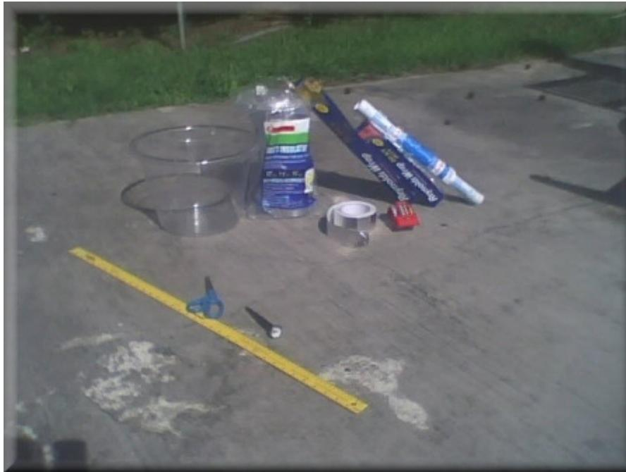
Figure 3. Tools and materials used to make a PanCooker. From left to right: yard stick, scissors, meat thermometer, 12-quart jumbo ice bucket, self-adhesive HVAC duct insulation, 12 inch and 18 inch rolls of heavy duty aluminum foil, 18 inch roll of self-adhesive clear plastic contact paper, aluminum foil tape and clear packing tape.
