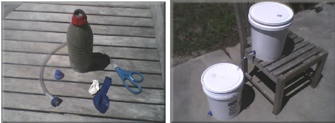
**Figure 4.** Preparing the bottle and spigot for connection to a 5-gallon turbid water treatment setup. A hygiene setup includes closed lids with vinyl tubing connection.
