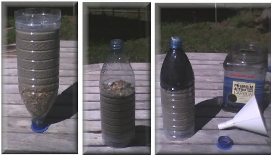
**Figure 3.** Making a binary concrete-carbon filter in stages.
