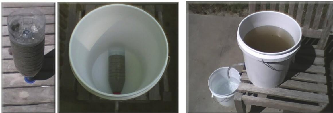
**Figure 1.** Porous concrete bottle filter used with a 5-gallon bucket for turbid water treatment.
