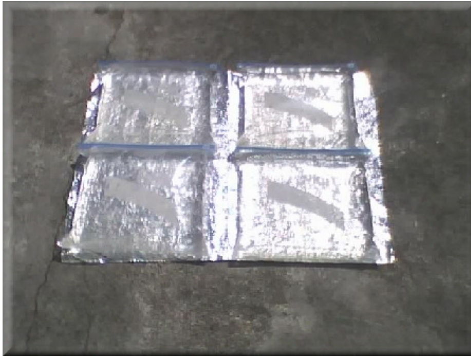
Figure 2. 12-quarts of hazardous water being treated by 4 handmade SODIS bags on a sheet of aluminum canvas . This amount of water will satisfy the daily needs of most households. The setup in this picture costs about $2-dollars.
