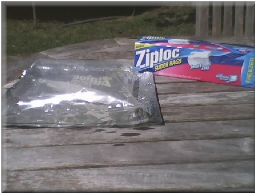
Figure 1. Modified 1-gallon freezer bag called into SODIS service.
