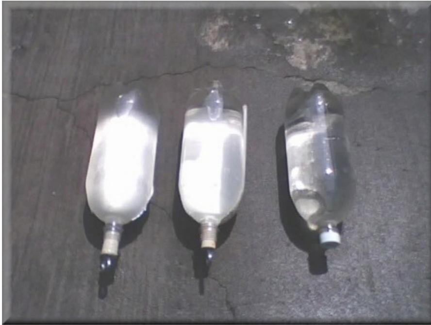
Figure 6. Comparison of jacketed aluminum and white plastic SODIS bottles (left) with a basic SODIS bottle (right).
