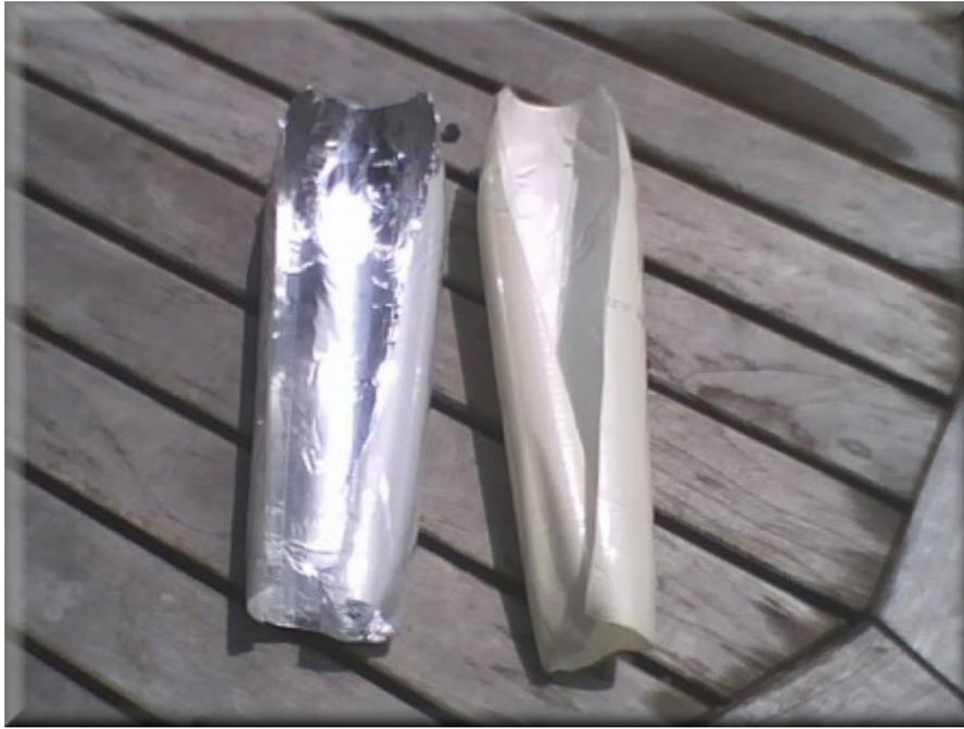
Figure 9. Completed Solar Jackets - aluminum foil tape (left) and white plastic duct tape (right)
