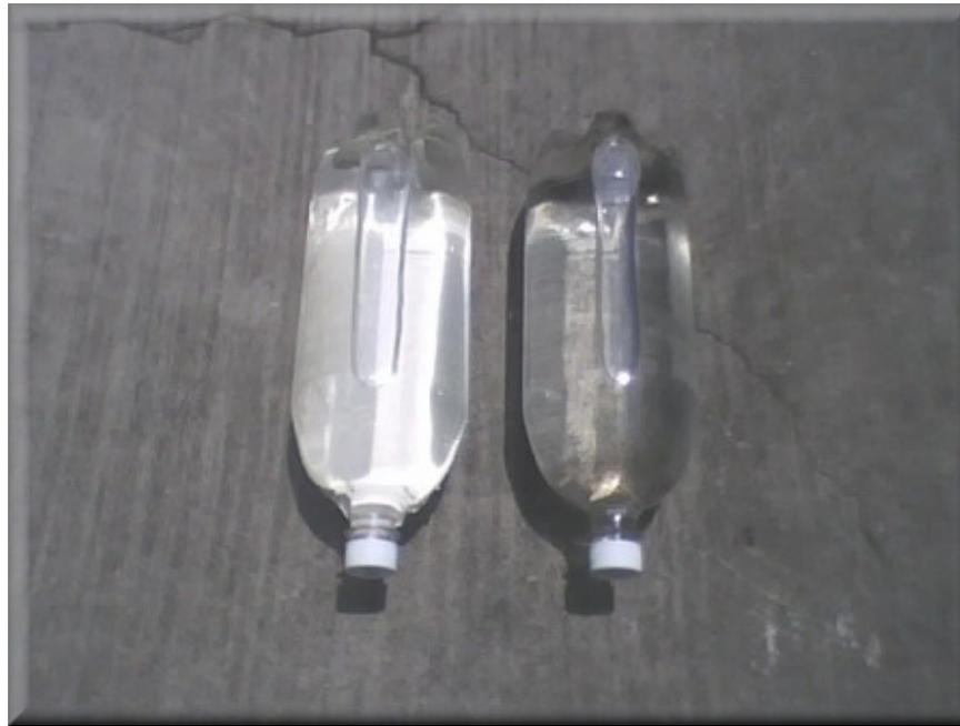
Figure 5. Taped SODIS bottle (left) compared to basic SODIS bottle (right).
