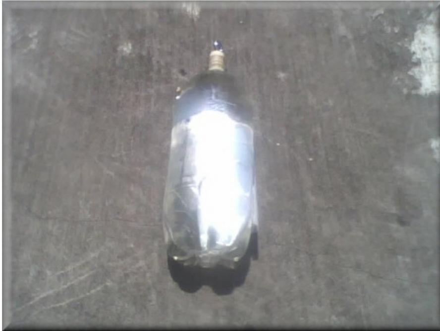
Figure 3. Amplified SODIS method = water bottle + solar jacket + bottle stopper + 6 hours of sunlight
