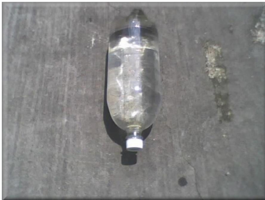
Figure 1. Basic SODIS method = water bottle + 6 hours of sunlight.
