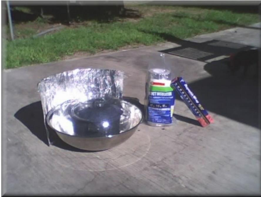
Figure 4. Sun Bowl with an additional back reflector made from 12 inch self-adhesive HVAC duct insulation and 12 inch heavy duty aluminum foil (optional).
